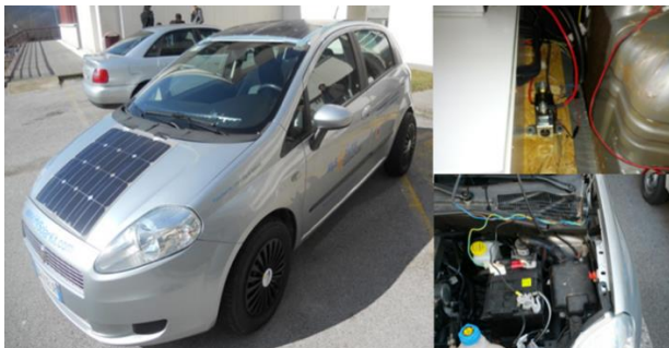
Figure 2 - HySolarKit installed on a FIAT Grande Punto and some wiring details.
