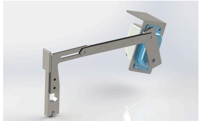
Fig. 5: CAD drawing of the mechanism used to provide autonomous control to the SAE vehicle's brakes.
