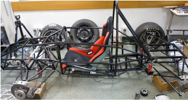
Fig. 2: Formula SAE-Electric frame.
