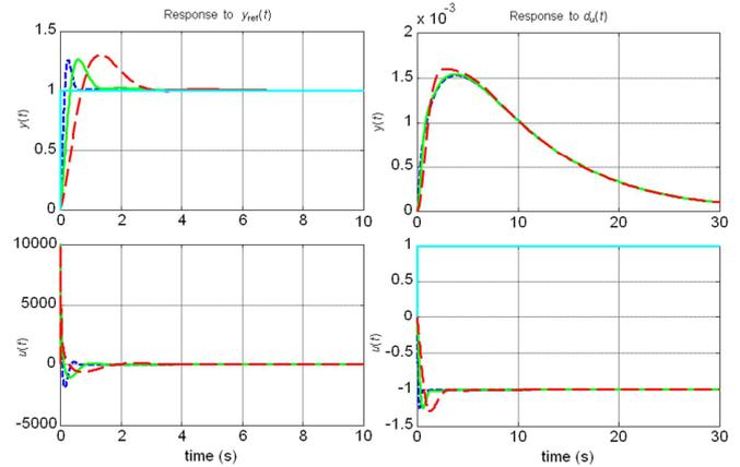
Fig. 11. Closed-loop step responses with the CRONE controller for the 3 values of  $\tau$ :  $\tau = \tau_{nom}/3$  (---),  $\tau = \tau_{nom}$  (—) and  $\tau = \tau_{nom} * 3$  (- -)
