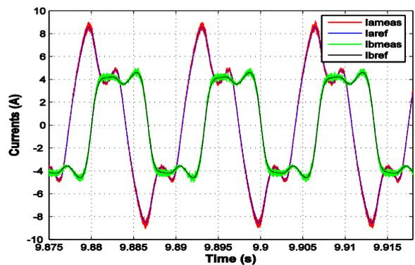
Fig. 9. Currents in the phase a and b under fault operation
