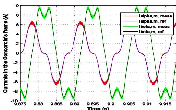
Fig.11. Currents in  $\alpha_m \beta_m$  frame under fault operation
