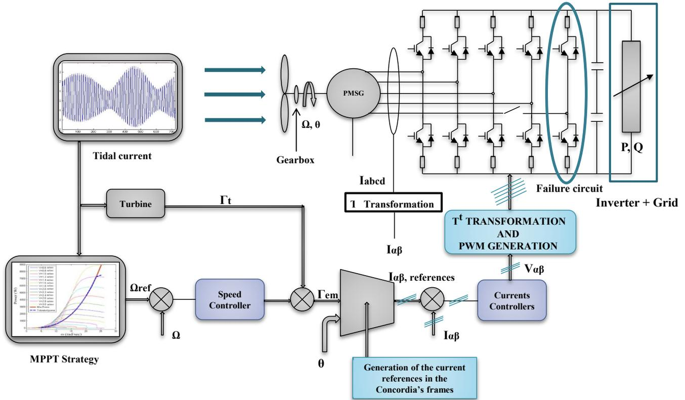
Fig. 1. Control scheme of the 5-Phase Permanent Magnet Synchronous Generator under Fault Operation
