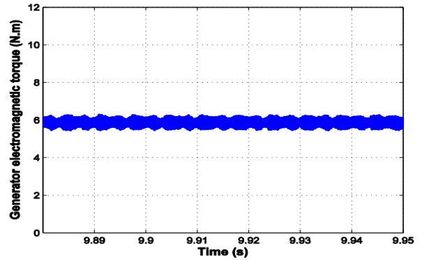
Fig. 6. Generator Torque under fault operation
