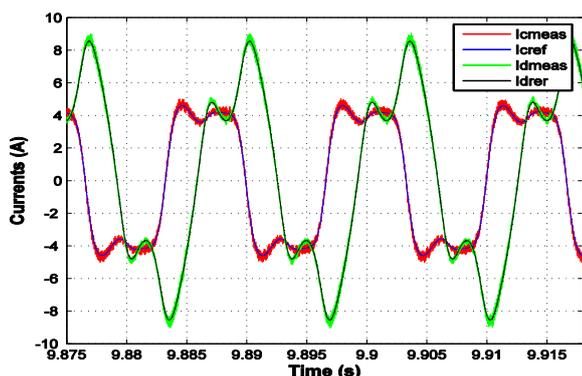
Fig.10. Currents in the phase c and d under fault operation
