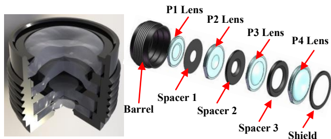
Fig. 1 Sample of lens module and its structure
