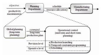
Fig. 3. The 2nd level of HMRPS
