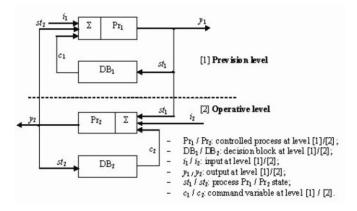
Fig. 4. Two-loop control model for the Operational control
