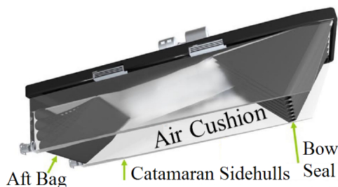
Fig. 1. SES hull, bag and bow seal (photo: Umoe Mandal)
