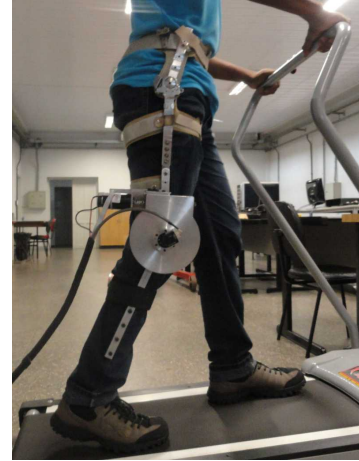
Fig. 5. Rotary SEA attached to a knee orthosis
