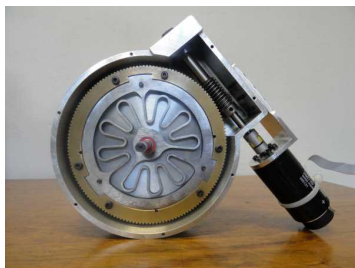
Fig. 4. Rotary Series Elastic Actuator
