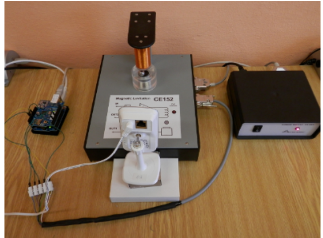
Fig. 5. Laboratory model of magnetic levitation
