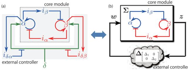
Fig. 2. Switchable memory circuit (a) is transformed to feedback form (b)
