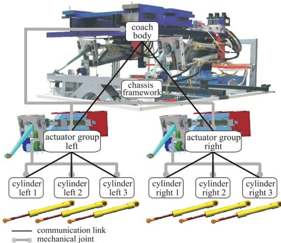
Fig. 1. Structure of the half-vehicle test rig.
