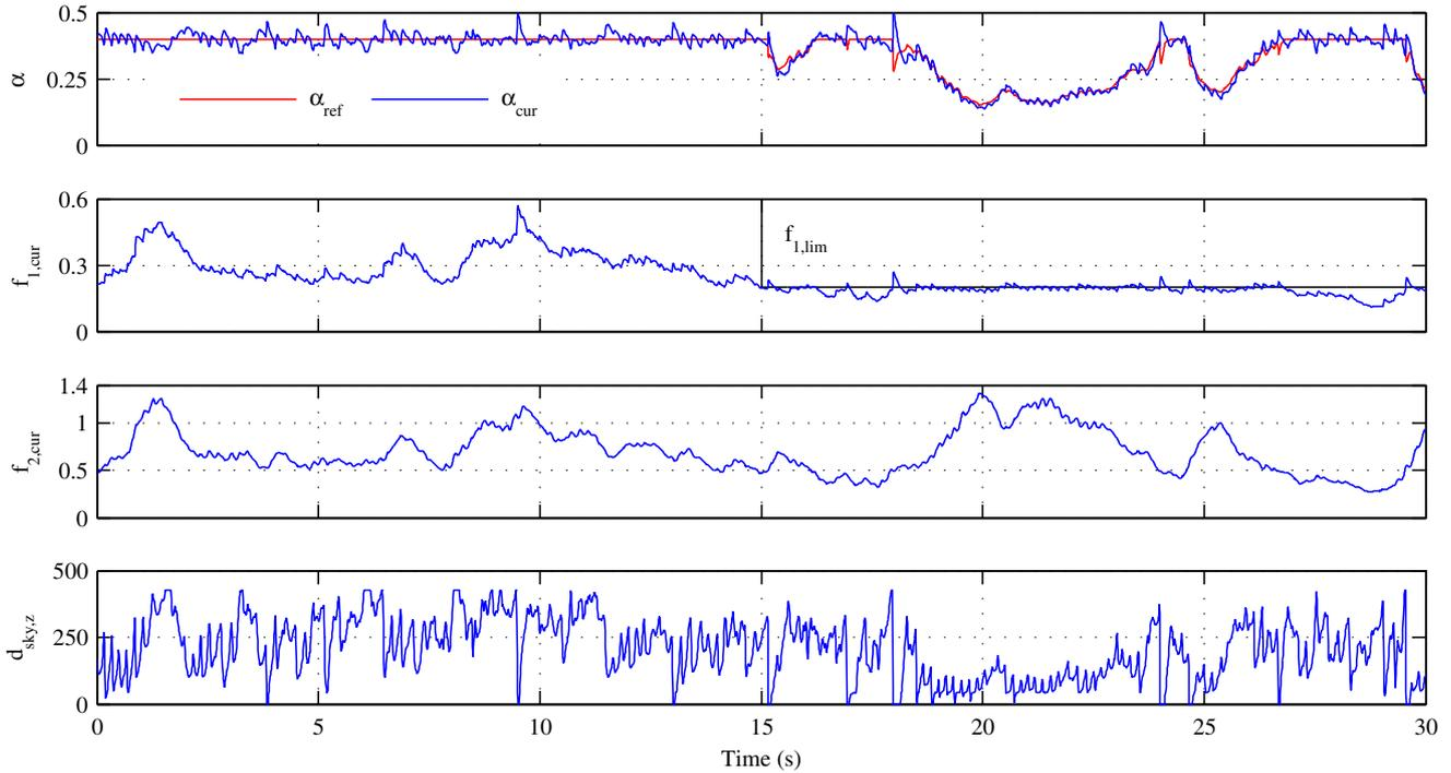
Fig. 7. Test rig results of the reference and current relative weighting  $\alpha_{ref}$  and  $\alpha_{cur}$ , the approximated objective values  $f_{1,cur}$  and  $f_{2,cur}$ , and the sky-hook controller parameter  $d_{sky,z}$  in vertical direction.
