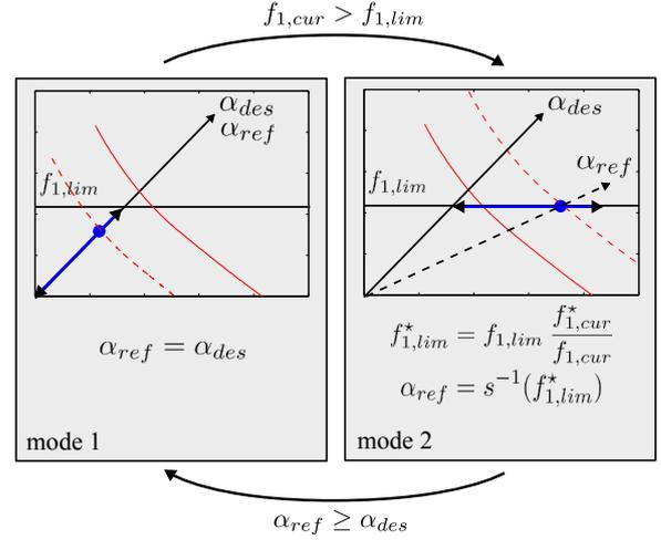
Fig. 6. Switching logic for the  $\alpha_{ref}$  value.
