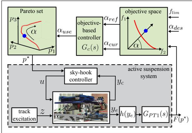
Fig. 4. Structure of the objective-based controller for the active suspension system.
