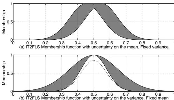
Fig. 2. Gaussian IT2FL Membership functions. (a) IT2FL MF with fixed variance. (b) IT2FL MF with fixed mean.
