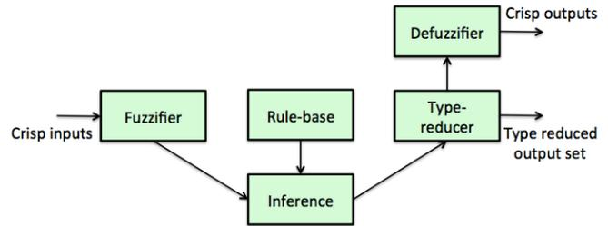
Fig. 3. Structure of an IT2FLS.
