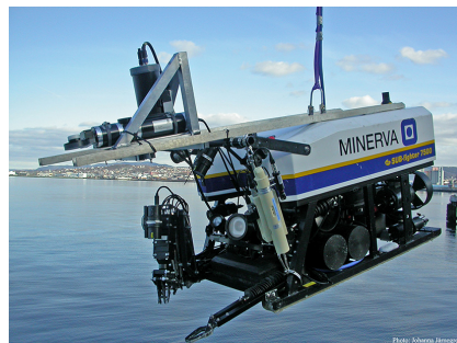
Fig. 1. ROV Minerva 1 , a SUB-fighter 7500 ROV from Sperre A/S. Photo: Johanna Järnegen
