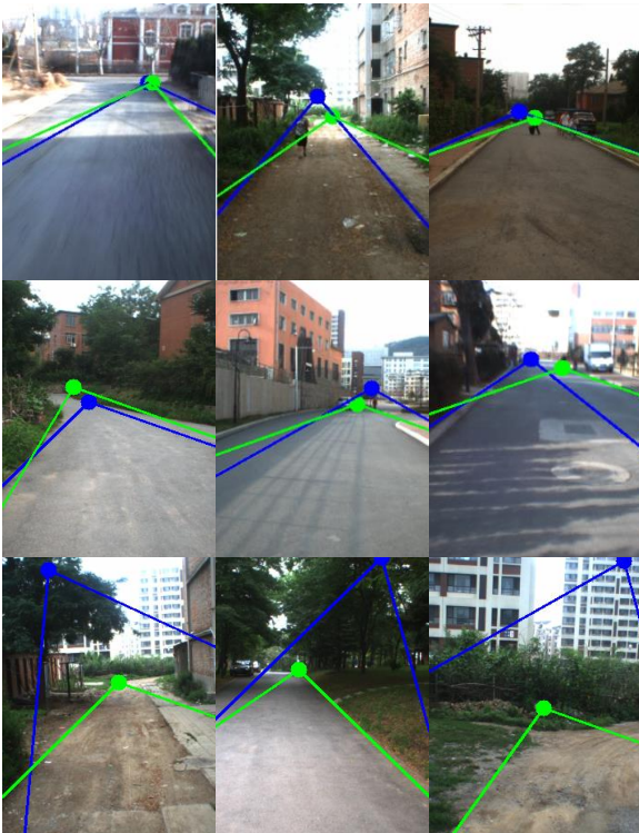
Fig. 11. Some experimental results of road detection.
