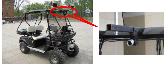
Fig. 8. Smart-Cruiser, a home-developed UGV equipped with multiple lasers and monocular cameras. A FlyCapture Flea2 camera is mounted on the front top of our UGV platform.
