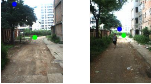
Fig. 6. Comparison of vanishing point detection. The blue point is detected by Kong et al. while the green one is detected by our method, respectively.
