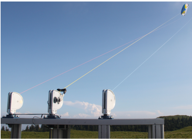
Fig. 1. Lead-out sheaves of the Swiss Kite Power prototype while flying a three line kite.
