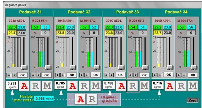
Fig.8. SCADA mimics of Air Control of the Coal Mills
