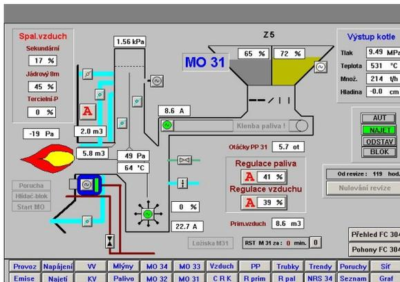
Fig.7. SCADA mimics of Coal Mills & Feeder
