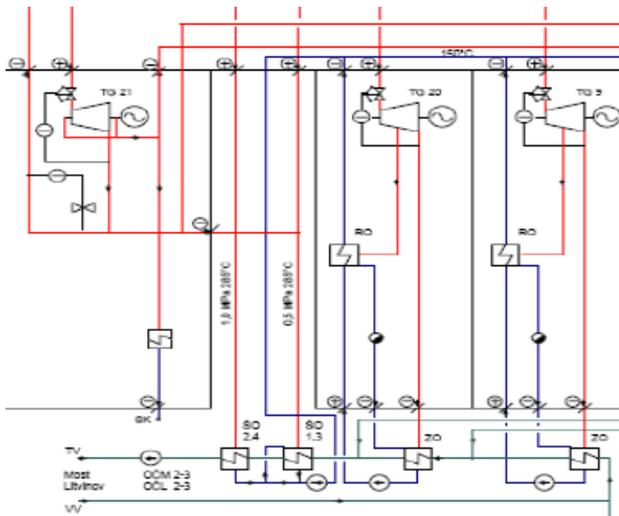
Fig.10. Relevant part of the technology scheme of central energy source
