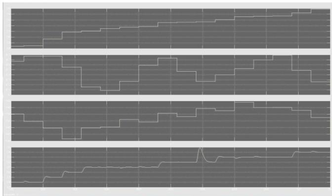
Fig.14. Overview of input values read from ORACLE and output values: order from the top: desired temperature  $T_z$ , return temperature  $T_{vv}$ , circulating water flow rate  $M$ , the output water temperature  $T_v$
