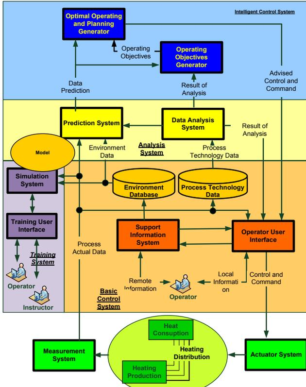
Fig. 1. The scheme of Smart Grid of district heating supply system with its control and training systems
