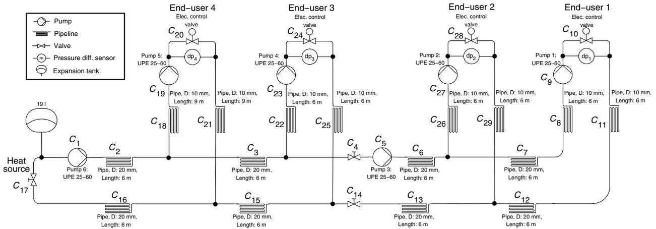
Fig. 3. Sketch of the hydraulic network used in the experiments.
