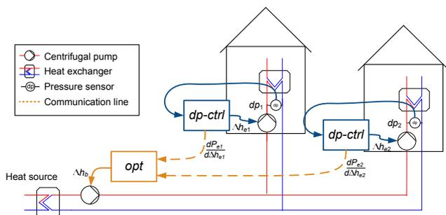
Fig. 2. A sketch of a small District Heating System with distributed optimization control.
