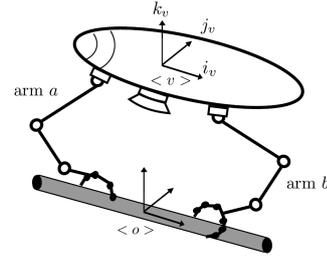
Fig. 6. Dual arm configuration with the relevant frames
