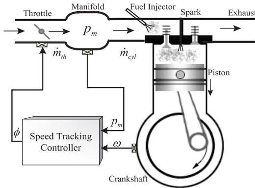
Fig. 1. The general structure of engine speed controller
