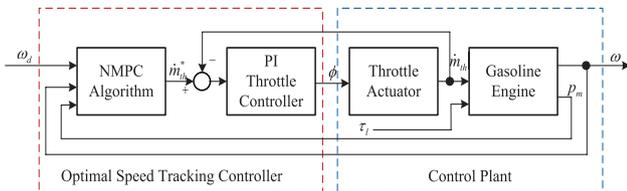
Fig. 2. The block diagram of the control scheme
