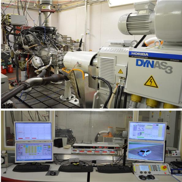
Fig. 5. The gasoline engine test platform
