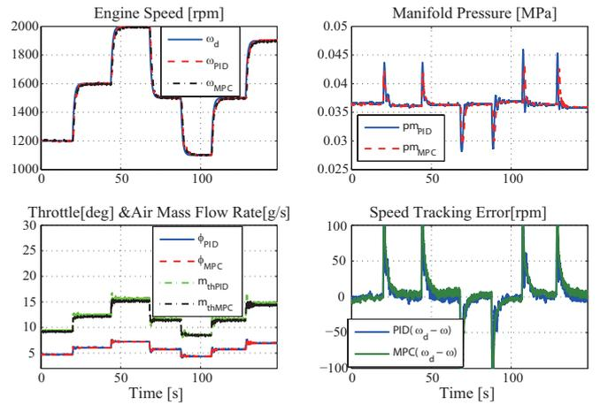
(a) The overall control effect for step test
