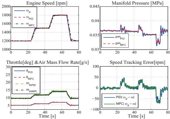
(a) The overall control effect for ramp test
