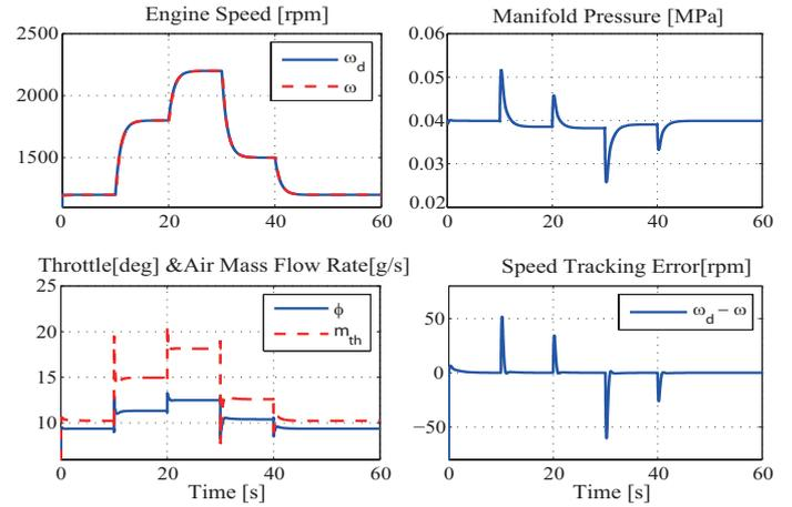
Fig. 3. Simulation results with step command tests
