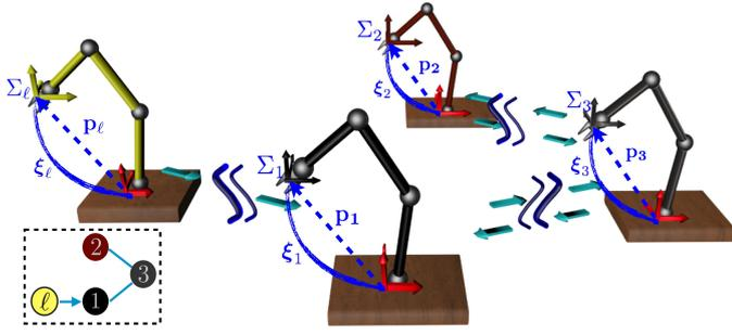
Fig. 1. Example of a robot network and the graph representing the interconnection
