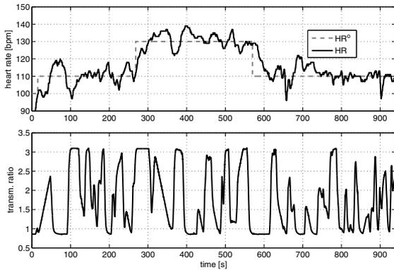
Fig. 8. Tracking performance of the SOSM controller.
