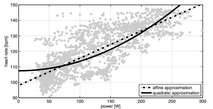
Fig. 5. Measured power/heart rate steady-state characteristic (dots), affine and quadratic approximations.
