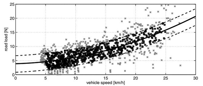
Fig. 2. Identification of the overall friction forces acting on the bicycle.
