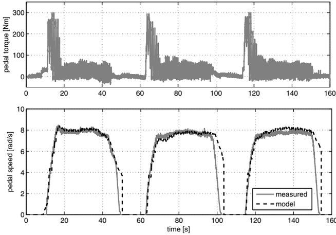
Fig. 3. Longitudinal dynamics model validation.
