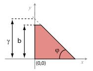
Fig. 3. The model of the tooth (top part of the *pCell*)
