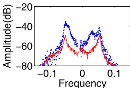
Figure 6: Measured FRF of the BLA (blue), and its standard deviation (red). Observe that the amplitude characteristic is not symmetric around the origin.
