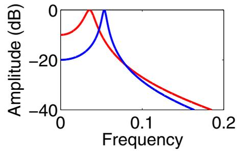
Figure 4: The transfer functions  $R$  (red) and  $S$  (blue) of the WH-system.
