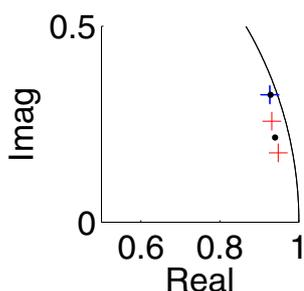
Figure 7: The estimated poles and their complex conjugates (only the first quadrant is shown). The black dots are the pole positions of the  $R,S$ -dynamic systems. The blue poles ( $S$ -system) did not shift, while the red poles ( $R$ -system) show a clear shift.
