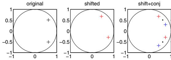
Figure 3: Shifted poles. Left: original poles; Middle: shifted poles; Right: shifted and conjugated poles. .
