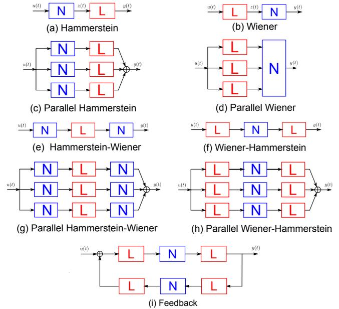
Figure 1: Examples of block-oriented nonlinear model structures.
