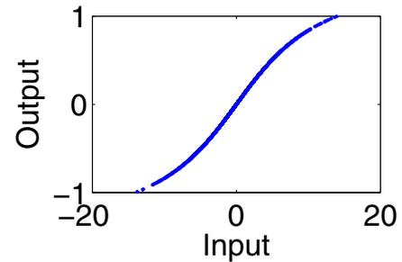
Figure 5: Static nonlinearity of the WH-system. .
