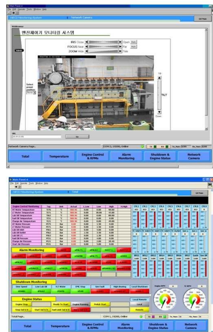
Fig. 14. Engine monitoring system
