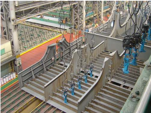
Fig. 6. Automatic panel welding robot system
