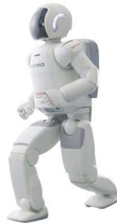
Figure 6: The Honda humanoid robot ASIMO is capable of both walking and running movements.
