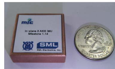
Figure 5: A Miniaturized ( 30 \times 30 \times 8 \text{ mm}^3 ), mountable Printed Circuit Board (PCB-mountable), 3-axis inertial measurement unit (IMU) complete with signal processing MCU and serial communication (the unit has integrated MEMS accelerometers and gyroscope as well as signal readout SOC inside.) The IMU can be used for motion control in automobiles, robots, and other motion systems.
