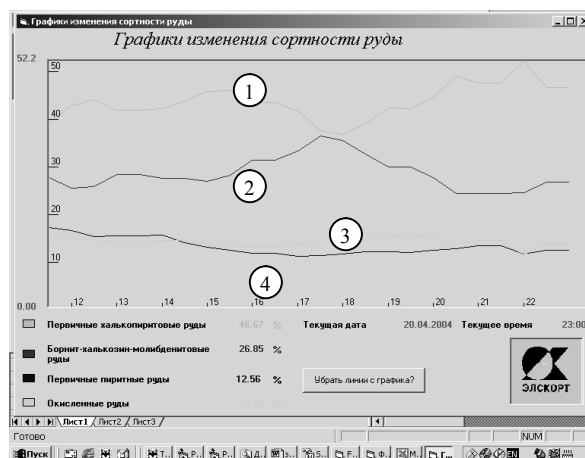
Fig. 7. Results of estimation of processed ore grade at “Erdenet” concentrator 1 - Primary chalcopyrite ores; 2 - bornite-chalcocite-molybdenite ores; 3 - primary pyrite ores; 4 - oxidized pyrite ores
