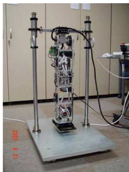
Fig. 1. Newly designed foot and landing leg platform
