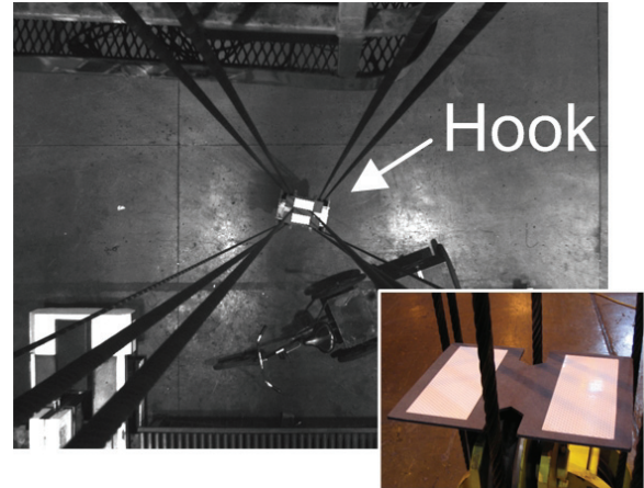
Fig. 7. Image captured and processed by the machine vision system (large photo). Close up photograph of the fiducials mounted on the hook (sub photo).
