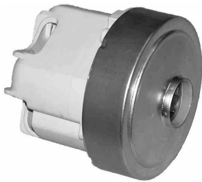
Fig. 1. The vacuum cleaner motor has a plastic housing, which enables smaller dimensions and impedes copying by the competition. The basic characteristics are: nominal speed-800Hz, voltage-230V, power-1.6kW.
