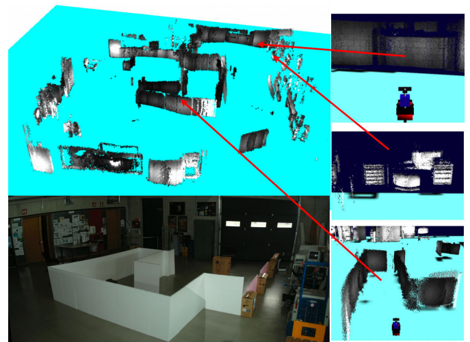
Fig. 10. Picture and global 3D map of test environment. On the right side three different viewpoints are shown (exocentric close, egocentric, exocentric far).
