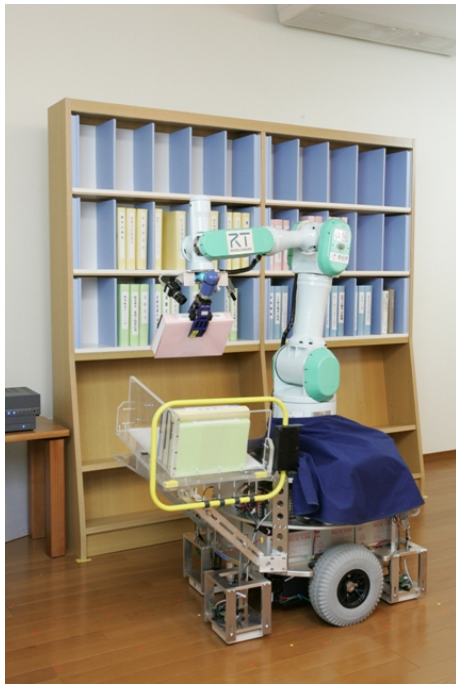
Fig. 2. The librarian robot system, the intelligent floor, and the intelligent bookshelf.
