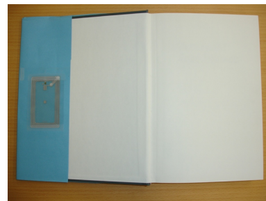
Fig. 8. A book with an RFID tag which gives the link information for a robot to access the Web DB.
