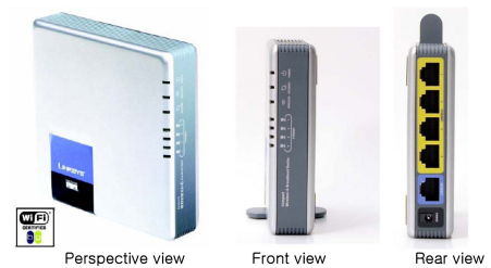
Fig. 4. Wireless access point
