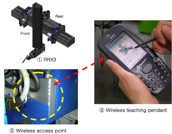
Fig. 3. RRX3, Wireless access point, and PDA TP
