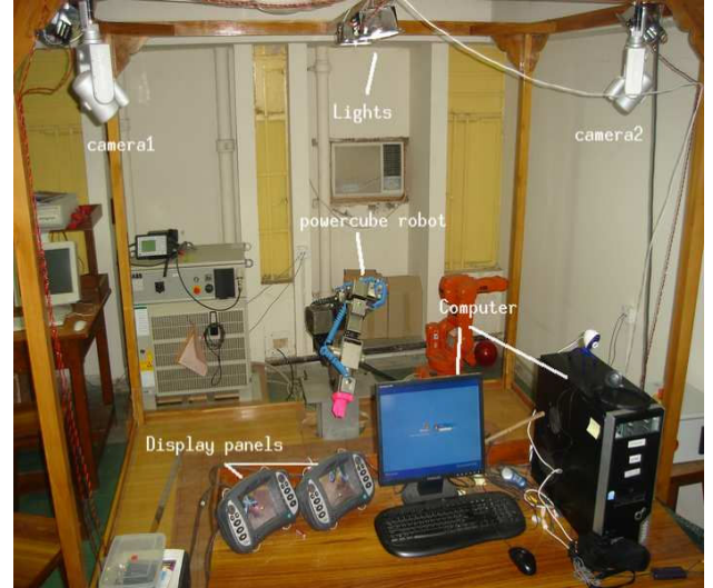
Fig. 1. Experimental setup with stereo-vision cameras and PowerCube TM
