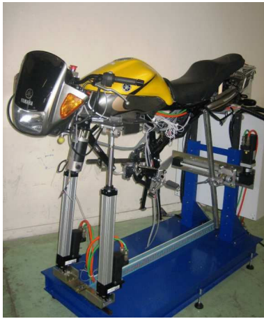
Fig. 8. Constructed riding motorcycle simulator
