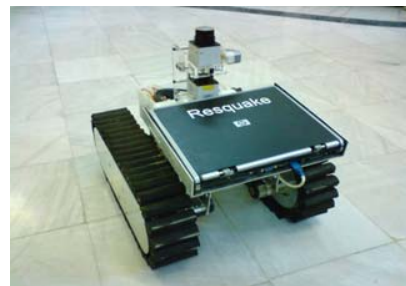
Fig. 4. Melon, the mobile robot equipped with low range laser scanners
