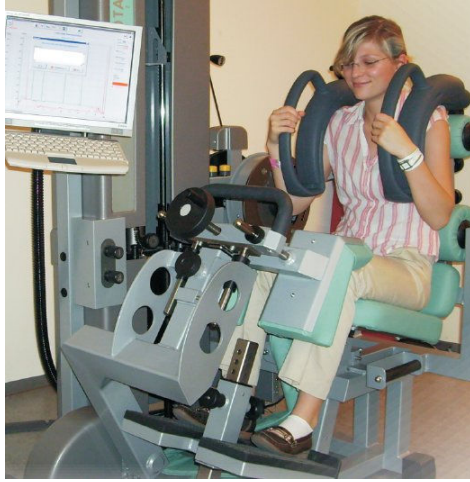
Figure 1. Device for measurement of the isometric contraction force of the lower back extensors (Total Trunk, Technogym).
