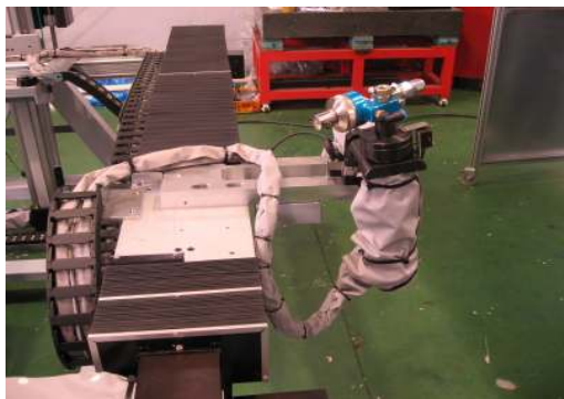
Fig.8 Painting reciprocator with five axes
