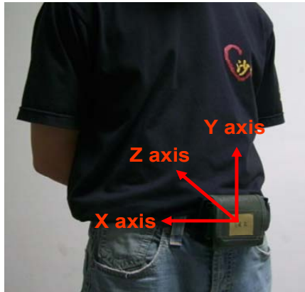
Fig. 3. Sensor axis of the human posture detection
