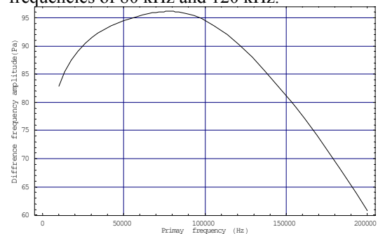
Fig. 2. Difference frequency generation with respect to the first primary frequency
