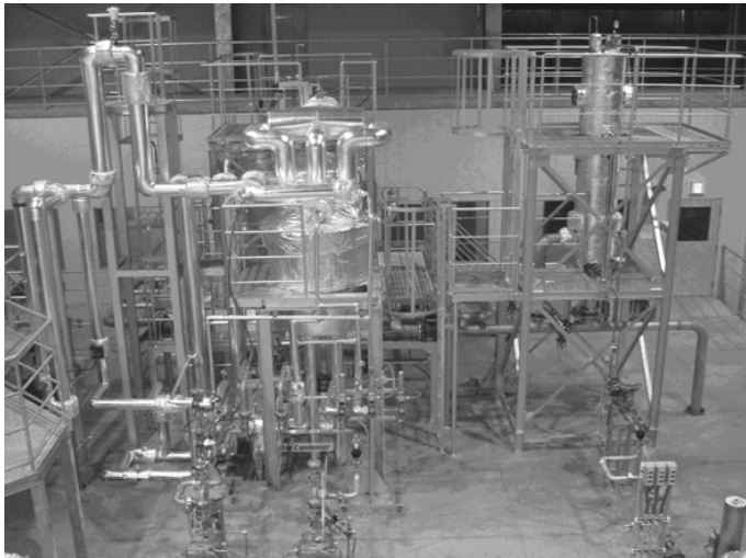
Fig. 2. Photograph of the experimental spray flash desalination plant (Ikegami et al [2006]).
