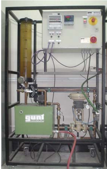
Fig. 8 – Water Level Plant, Process Control Lab. – Electrical Engineering Department, K. N. Toosi University of Technology
