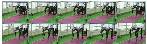
(b) Consecutive scenes of the trots at average velocity of about 0.5m/s.
