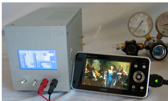
Fig. 5. Photograph of the fuel cell and battery hybrid system demonstrated at ISLPED 2007 design contest.
