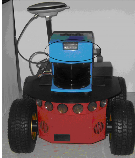
Figure 2: ActivMedia robot with 16 sonars and a rangefinder laser
