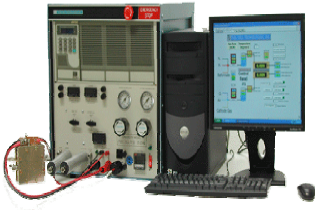
Fig.1 Fuel cell Test station
