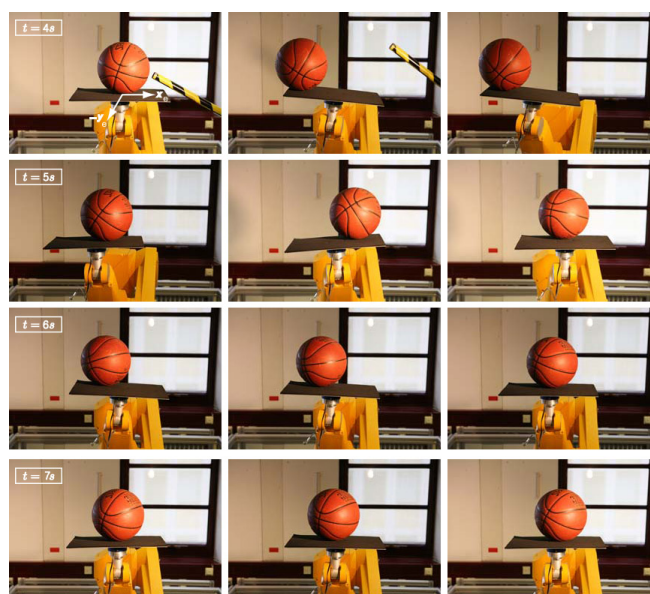
Fig. 2. Sequential snapshots of stabilizing a basketball against an external impact force at t = 4 s.
