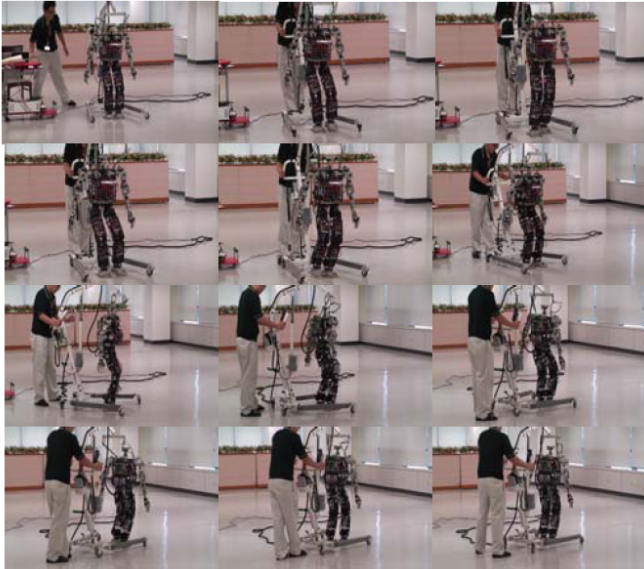
Fig. 7. J-turn walking of MAHRU-R on uneven office floor. uneven terrain and Fig. 8 shows that it can track the given CoM / ZMP trajectory very well.
