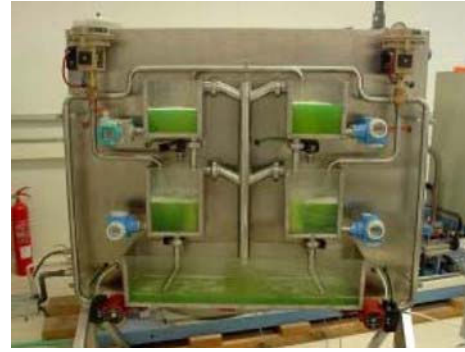
Fig. 3. Scale-model of the quadruple-tank process used to test the proposed method.
