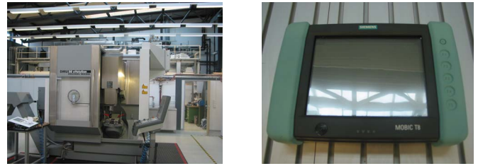
Fig 4. Experimental setup with 5-axis milling centre and mobile Personal Digital Assistant
