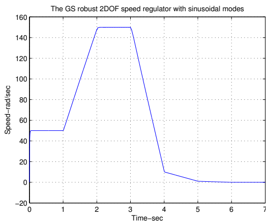
Fig. 5. Speed output with the GS robust 2DOF regulator.
